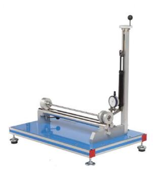
**Torsion Test Apparatus – Model KSM-097.** Torsion occurs when a moment or torque is applied to a rod or structural element, causing its transverse sections to twist around an axis normal to their plane. This results in tangential stresses similar to simple shear stresses. In industry, torsional stress is common in machine shafts that rotate and transfer motion.
